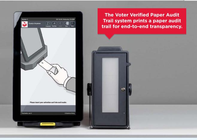
When used in the direct record electronic (DRE) configuration, the ImageCast® X can be paired with a Voter Verified Paper Audit Trail (VVPAT) thermal printer. Every electronic record stored on the ImageCast® X redundant memory has a corresponding paper record copy in the form of the VVPAT receipt.
