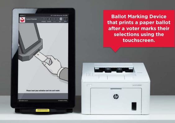
The ImageCast® X can be configured as a Ballot Marking Device (BMD), which is paired with a commercially available, compact laser printer that prints a summary of the voters selections. No votes are stored on the ImageCast® X when in the BMD configuration.
